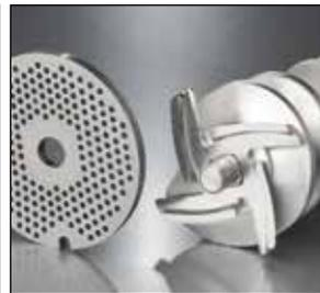
3. Attach the needed accessories (in this case: crossed-blade knife and grinding disc). Take the crossed-blade knife and attach it to the worm. The rounded side of the knife must face the worm when attaching it to the axis of the worm. Ensure the square opening of the crossed-blade knife fits over the four cornered shaft of the worm (picture C and D).
