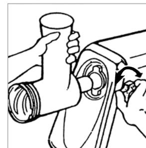
3. Loosen the screw plug on the right side of the mincer by turning it counterclockwise until you can take the worm housing out of the motor housing without any resistance (picture B).
