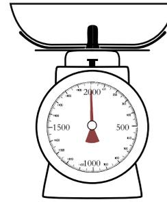
1. Turn the button until the red arrow on the measuring scale is pointing straight up, if you want to reset the value to "zero".
