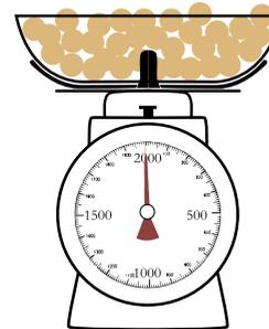
3. You can set the value back to "zero" by turning the button repeatedly until the red arrow on the measuring scale is pointing straight up. The weighing scale can remain filled.
