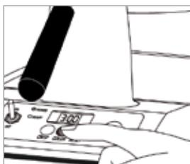
3. Push the toggle switch to on to begin the preheating process. The LED background displays blue and shows a default cooking time of 2:30.
