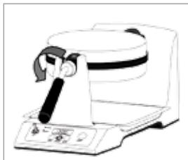
10. To remove the waffle, rotate the unit 180° counter-clockwise and lift the handle straight up. Once the waffles are cooked, carefully remove them; use a wooden or plastic spatula to remove waffle from the bottom plate. Make sure not to touch the cooking surface with sharp, pointed or metal objects; this could damage the non-stick surface. Use caution as the plate is extremely hot.
