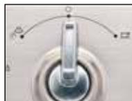
Make sure to position the selector switch to the ›Standby‹-position (middle) first. Press the ›on/off‹-switch and turn on the appliance. The power indicator lights red. During preheating the heating indicator lights red. Once the appliance is ready for operation the heating indicator turns off.
