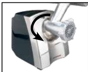
3. Firmly secure the worm housing in the opening for the drive shaft. The small end of the worm housing has to face the mincer. Incline the worm housing a little bit to the right, when assembling it. When the worm housing is fitted all the way into the opening of the drive shaft the release button sinks into the motor housing. Turn the worm housing counter clockwise until the shaft is facing upright.
