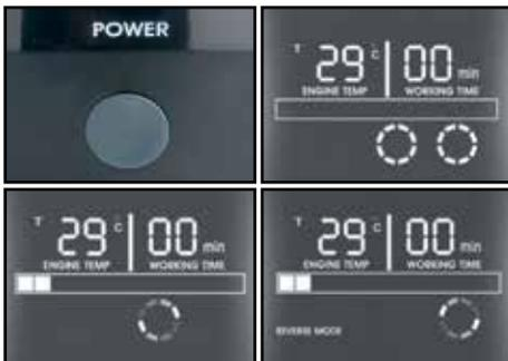
4. Press the power button on the back of the appliance. The display illuminates and you can see the motor temperature, working time and two circles.
