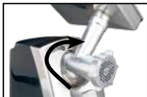
5. Remove the closing ring of the worm housing and take the inner unit (such as the worm, crossed-blade knife and grinding disc, Kebbe attachment, sausage attachment or cookie attachment) off the worm housing.
