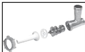
1. Take the worm housing into the right hand and insert with your left hand the worm inside the worm housing. The side of the worm with the plastic end has to face the worm housing when putting it inside the worm housing. If the worm is correctly assembled when the plastic end of the worm pokes a few millimetres out of the worm housing.
