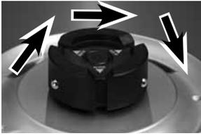
**ATTENTION:** Occasionally clean the drive coupling (see picture) with a damp cloth. Ensure the stainless steel balls of the basket adjustment are clean and free from dried on juice or pulp residue. After every fifth usage put some vaseline onto the balls of the adjustment.
