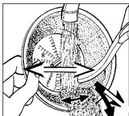
Using the cleaning brush, hold the filter basket under running water and brush from the inside of the basket to the outer rim. Avoid touching the small sharp blades in the centre of the filter basket. After cleaning the filter basket, hold it up towards a light to ensure the fine mesh holes are not blocked. If the holes are blocked, soak the filter basket in hot water with 10% lemon juice to loosen the blocked holes. Alternatively, wash the filter basket in the dishwasher.
