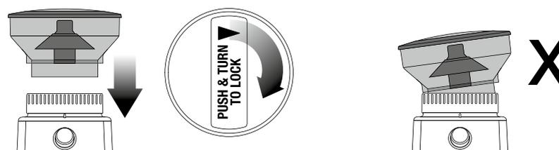
**NOTE:** You cannot lock the bean hopper with the bean hopper misaligned. The safety interlock will disable motor operation, if the bean hopper is not locked properly. In this case, the GRIND TIME dial will stay dark and the START/CANCEL button will be inactive even with the appliance connected to the power supply.
