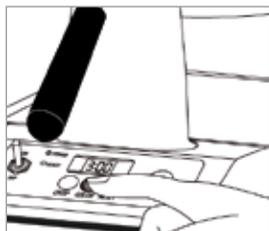
4. When the blue ready light is on and 3 beeps sound, preheating is finished. At that moment, one black point will be flashing in the LED display and a blue light illuminates under the colour button.
